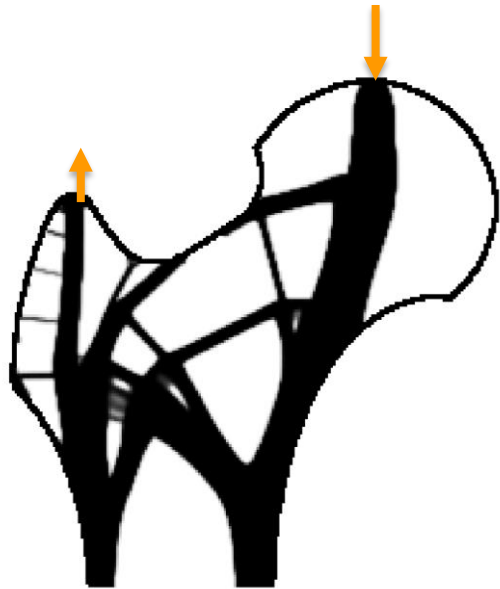
Infill by standard topology optimization
