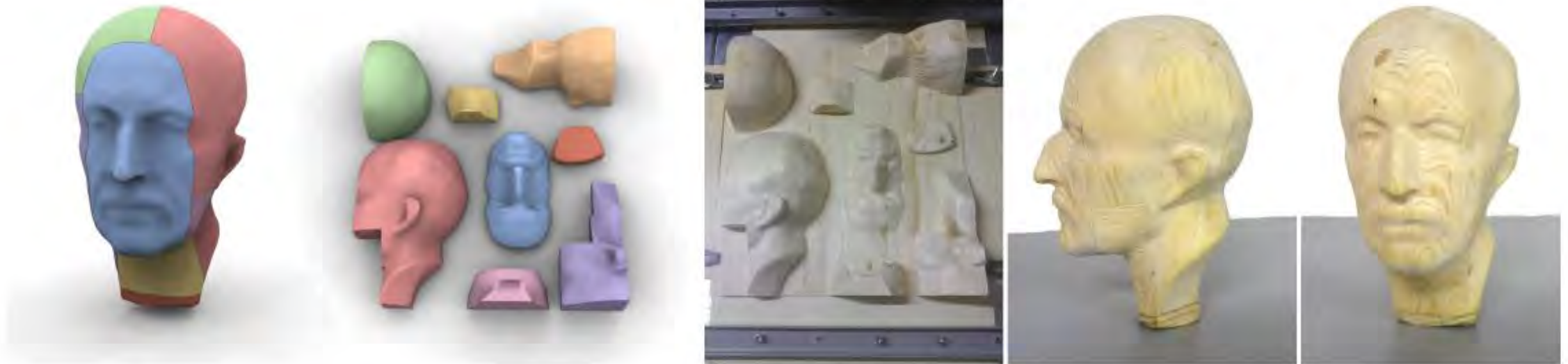
Fig. 1. We decompose general 3D geometries into height-field blocks (left), enabling their fabrication using single pass 3-axis CNC machining (right).
