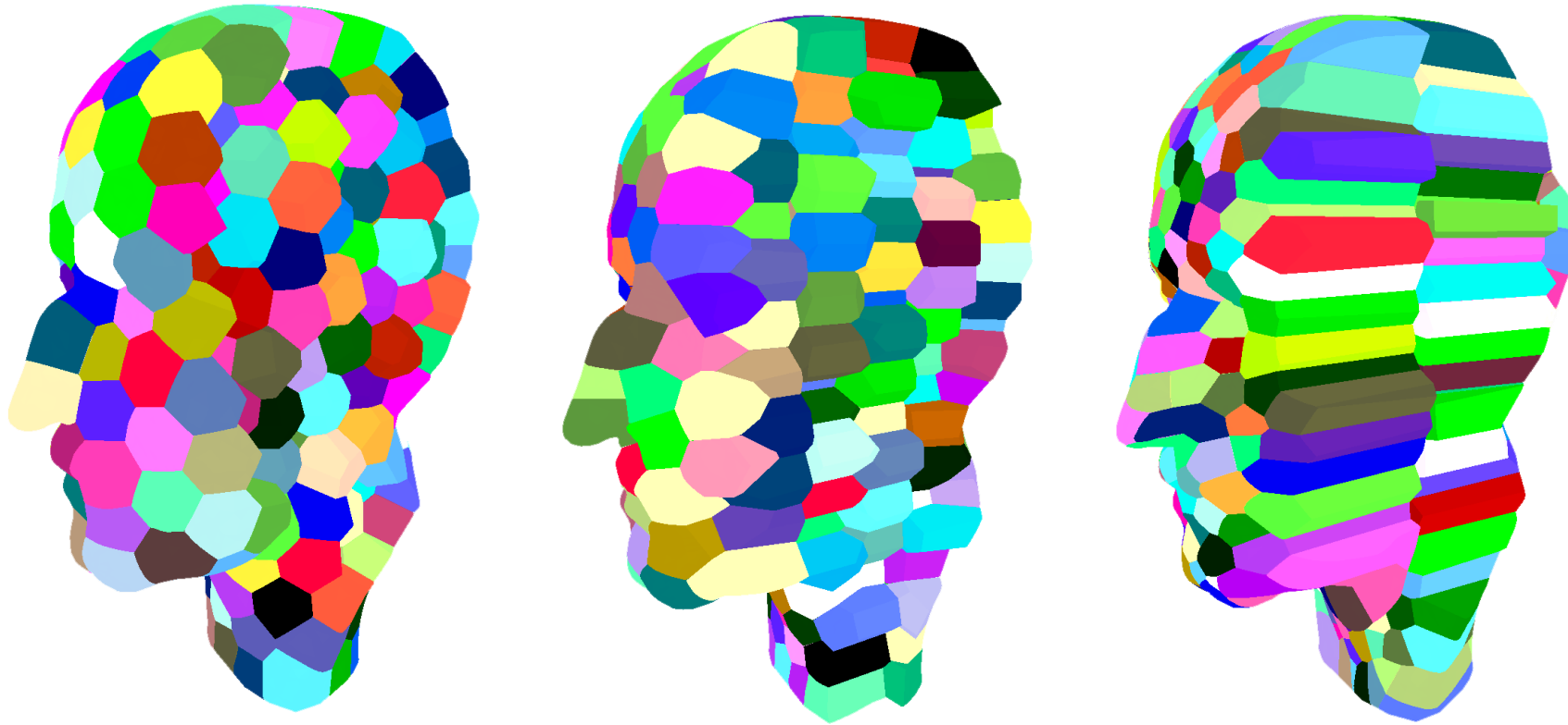
3D optimal power diagrams with increasing anisotropy Left: isotropic, middle: 2:1:1, right: 8:1:1
