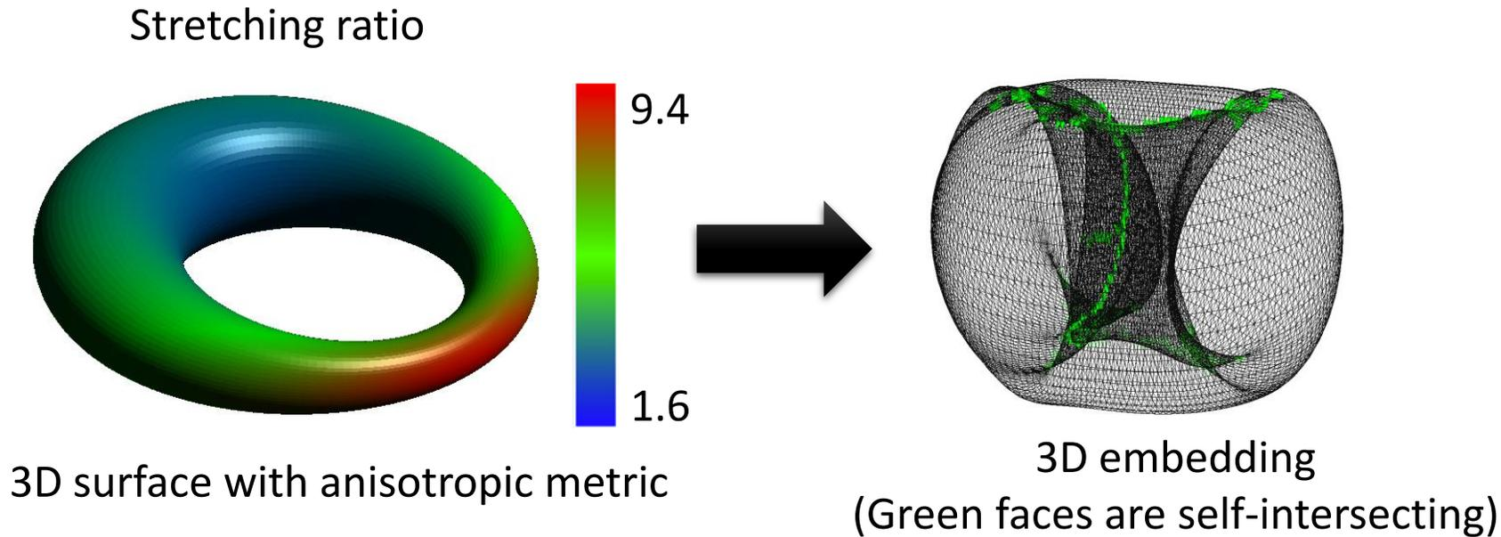
3D embedding result [Panozzo et al. 2014] of a Cyclide surface. There are 1146 self-intersecting faces out of total 21,600 faces as shown in green color
