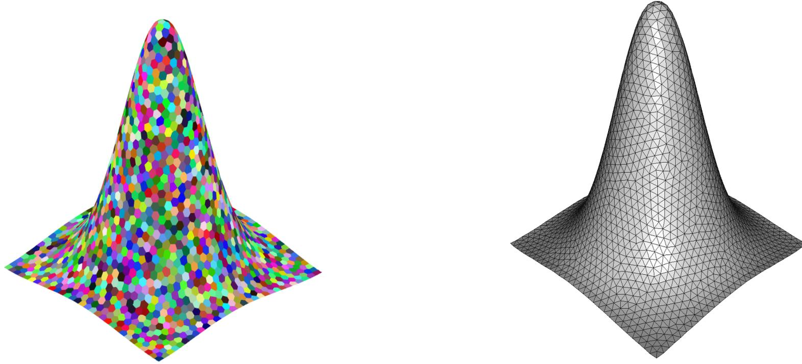
RVD and its dual mesh on a high-d embedded surface
