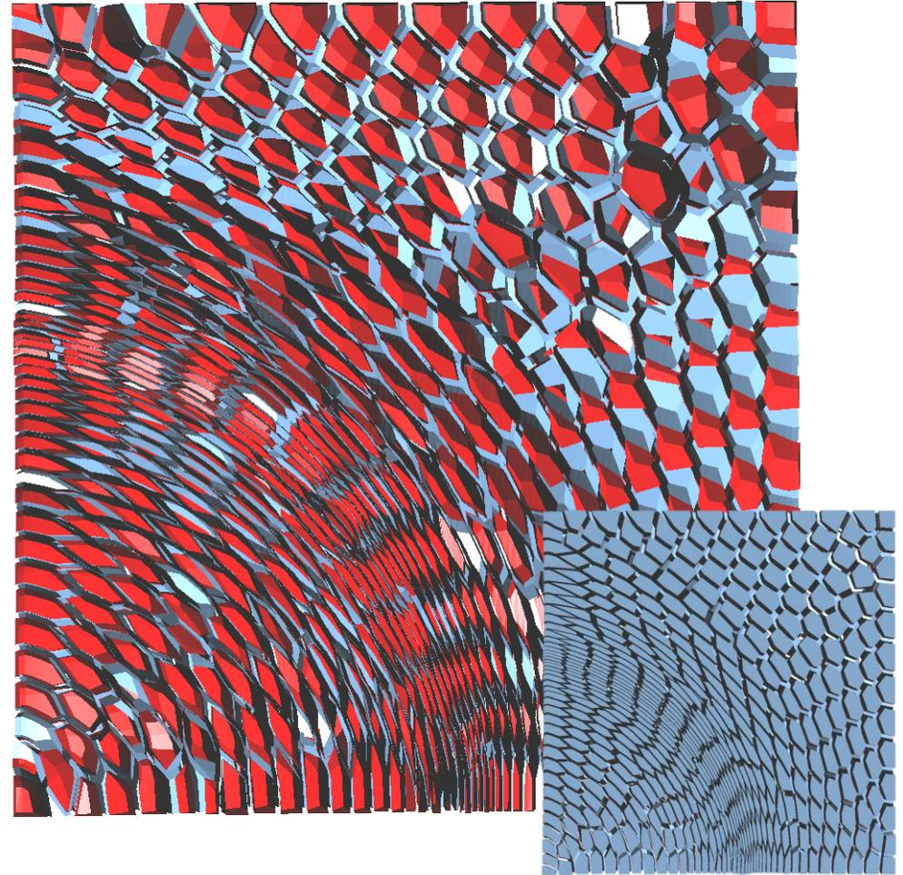
Stretching ratio  $\in [1, 20]$  defined by a highly nonlinear function with a cylindrical rotation field
