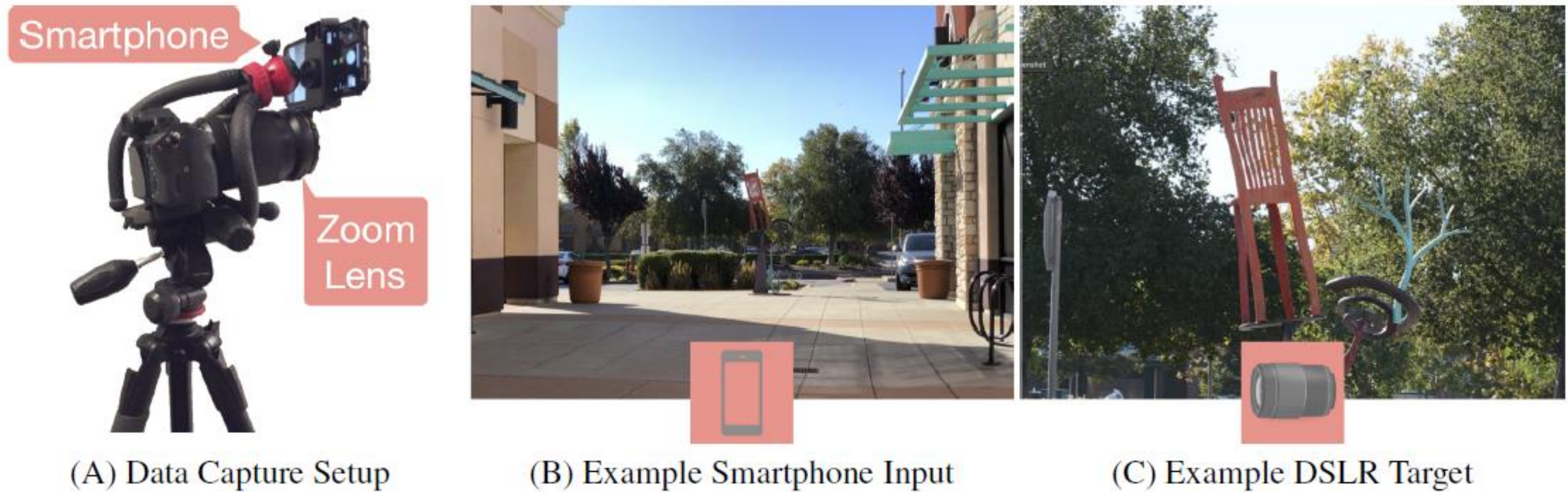
Figure 2: Smartphone-DSLR data capture and an example data pair.
