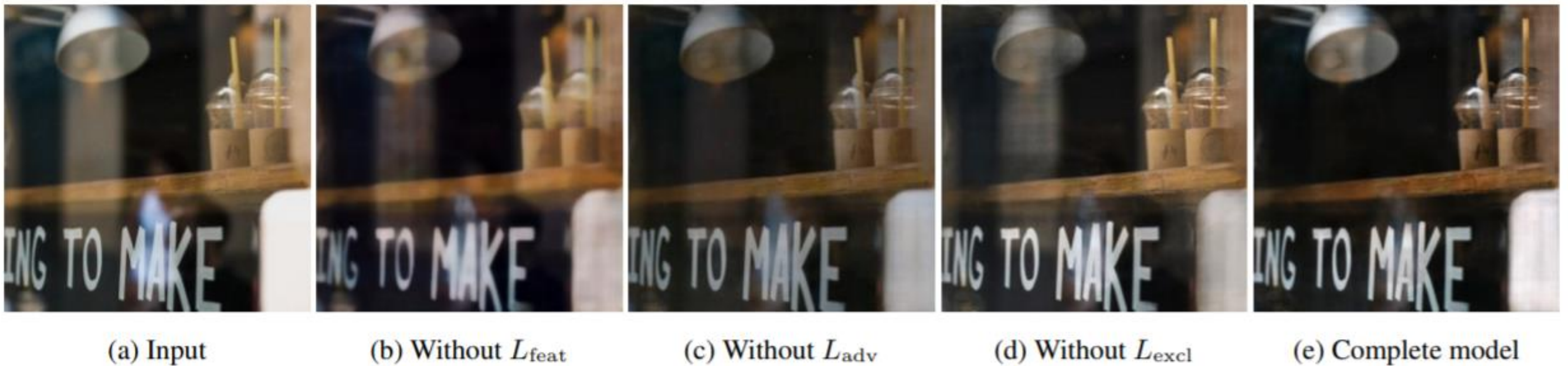
Figure 2: Visual comparisons on the three perceptual loss functions, evaluated on a real-world image. In (b), we replace L_{feat} with image space L^1 loss and observed overly-smooth output. (c) shows artifacts of color degradation and noticeable residuals without L_{adv} . In (d), the lack of L_{excl} makes the predicted transmission have undesired reflection residuals. Our complete model in (e) is able to produce better and cleaner prediction.
